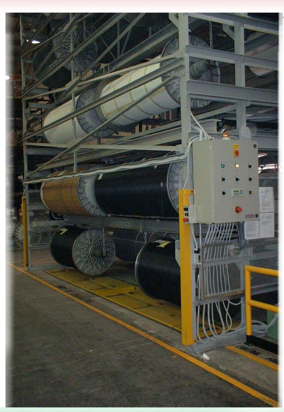
Transmission pulleys for V-shaped belts, for transmission between motor and reducer. The translation chains are designed for a high maximum tensile stress. The speed in the two directions of run is 7 meters/min. The stores have special pinions for the translation chain. The shafts are supported by single-bloc supports with spherical orientation.
